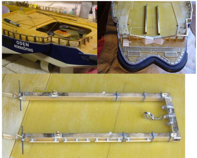
The aft anchorlight up-and-down-mechanic is ready.
